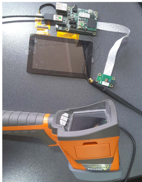
Fig. 5. Embedded system (top) and FLIR camera (bottom). Display is used only for debugging purpose. Embedded system has attached video camera which is used to provide complementary information
