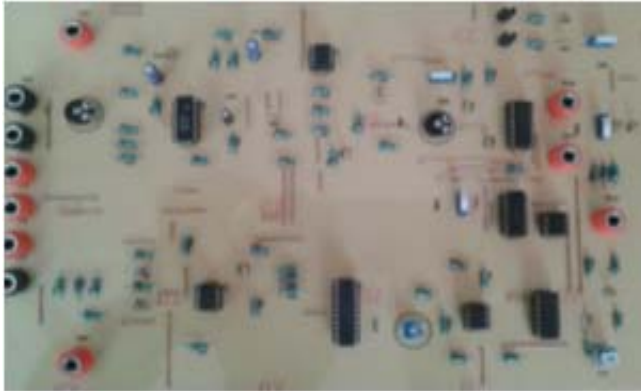
Fig. 6. The prototype board containing the QPSK modulator of the proposed digital modem.
