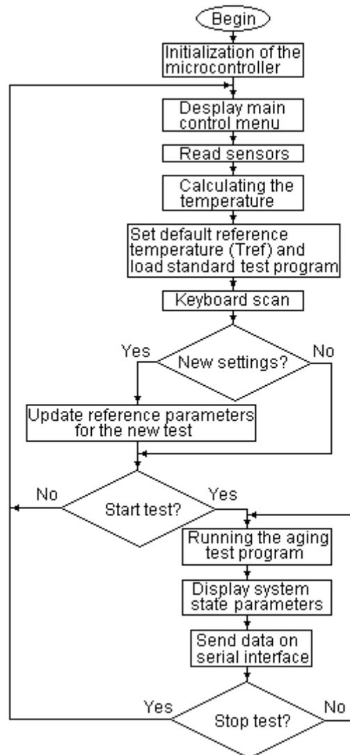
Figure 2. The state diagram of the main routine of the software application written for PIC16F777 microcontroller
