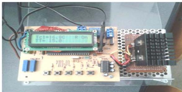
Figure 5. The implementation of the temperature control module, with high power MOS transistors mounted on the heat sink
