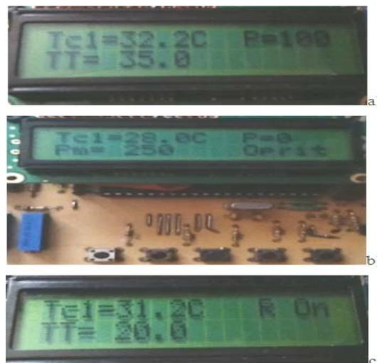
Figure 4. Few screenshots illustrating the operation of the system: a) the cooling state; b) the stand-by state; c) the heating state
