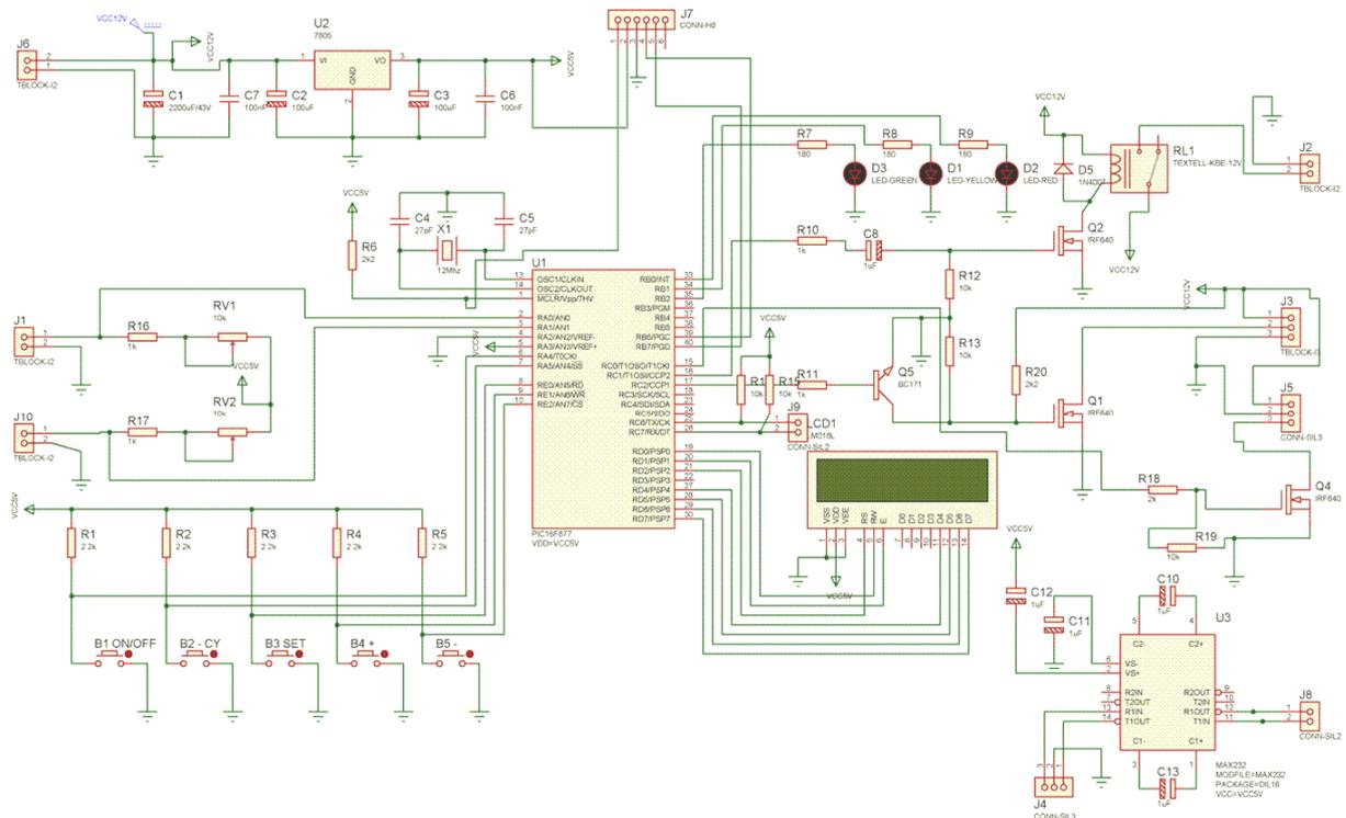
Figure 3. The schematic of the main module of the temperature control system used for accelerated aging tests on printed circuit boards
