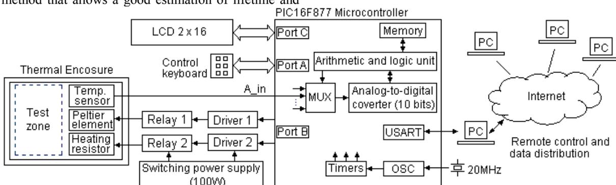
Figure 1. The simplified structure of the temperature control system used for accelerated aging tests on printed circuit boards
