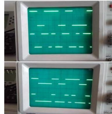
Fig. 8. The Manchester code in the figure above and RZ code in the figure below
