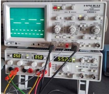
Fig. 6. Generated data and clock signals that are used for testing the correct operation of the line encoder.
