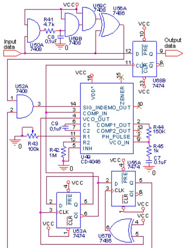
Fig. 3. The schematic of the synchronous decoder for Manchester line code.
