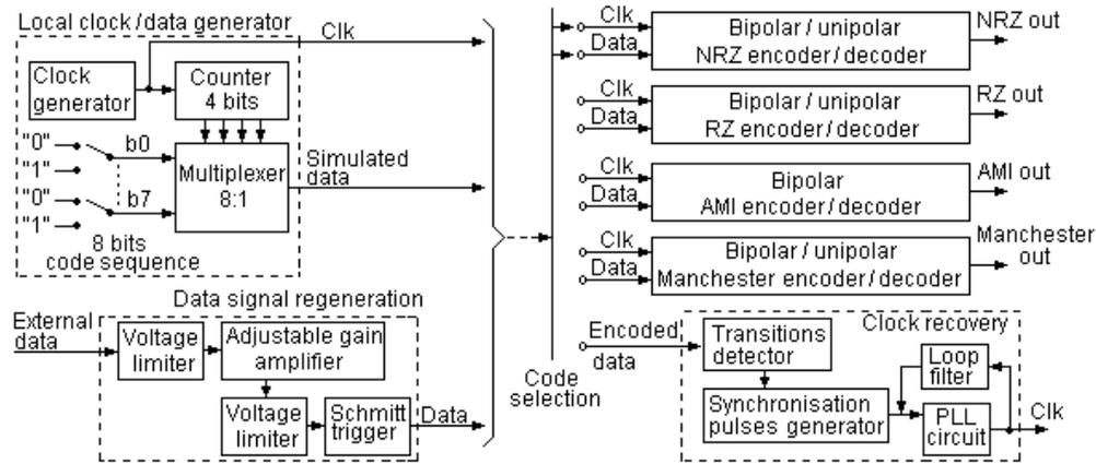
Fig. 2. The simplified block diagram of the line encoding/decoding system with serial data transmission for in-vehicle networking.
