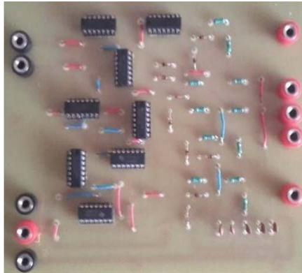
Fig. 7. The clock recovery circuit used for coherent decoding of the transmitted line codes.
