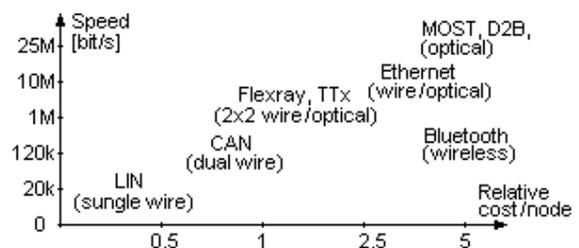
Fig. 1. Comparison between protocols used in automotive communications.
