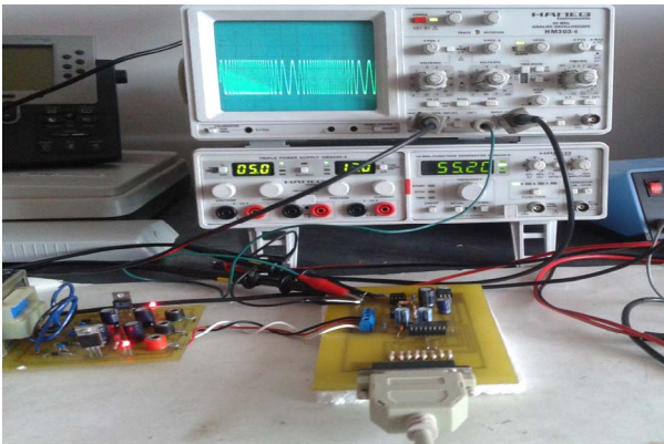
Figure 5. The experimental setup configured for synthesizing a frequency modulated signal that is visualized on a standard oscilloscope.
