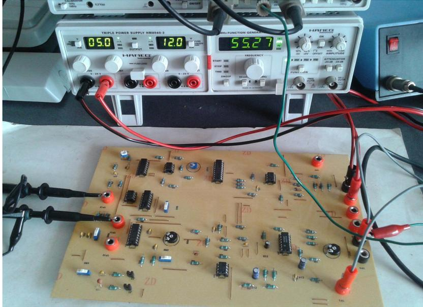
Figure 5. The experimental prototype of the conditioning and transmission module for resistive bridge sensors.
