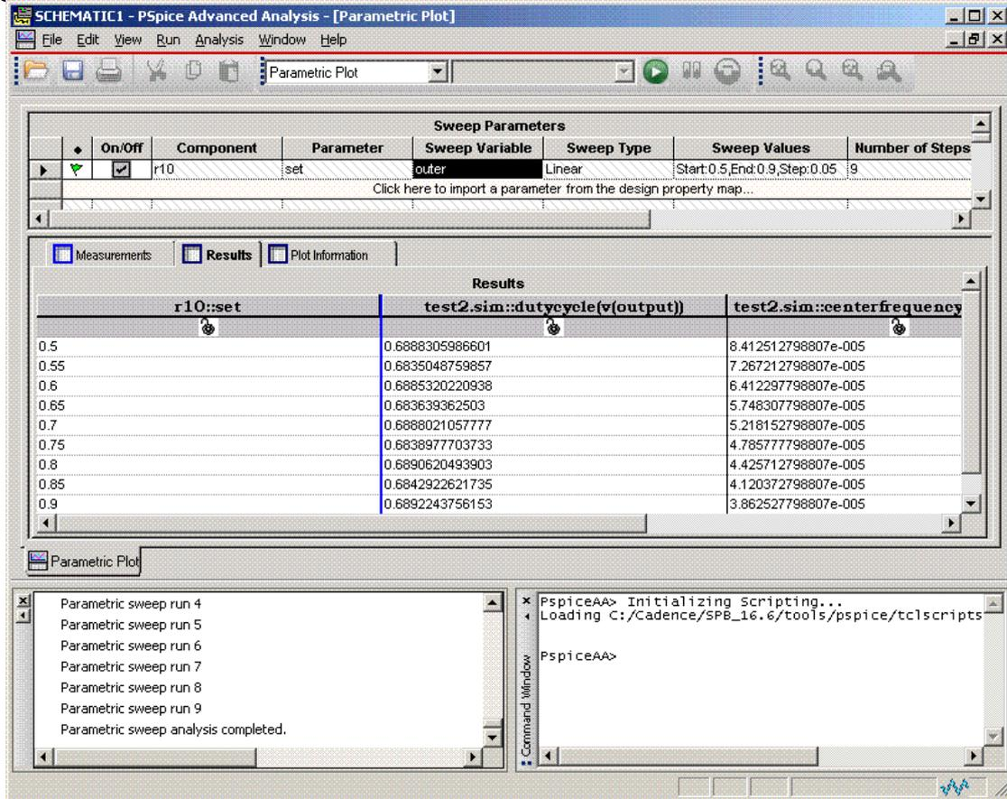
Figure 3. The parametric simulation results showing the values for the duty cycle and the frequency of the output signal generated by the module, considering the measuring bridge imbalanced due to a variations caused by resistor R10.
