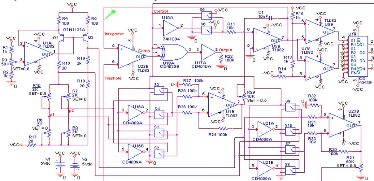
Figure 2. The electronic schematic of the module used for conditioning and transmission of signals from resistive bridge sensors.
