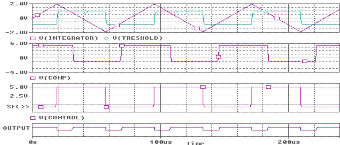
Figure 4. Sample waveforms obtained as a result of time domain simulation of the proposed module.
