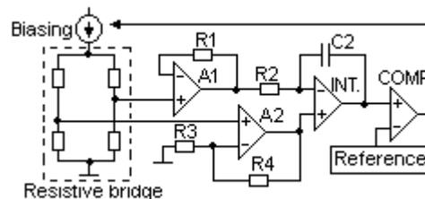
Figure 1. The principle of resistance-to-frequency converters.
