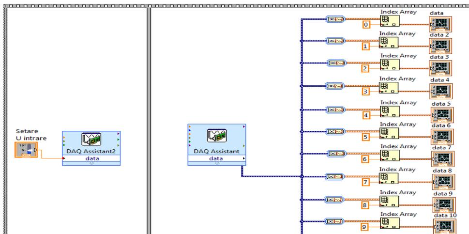
Fig. 4. LabVIEW code for waveform measuring of staircase digital voltmeter using NI-USB6212
