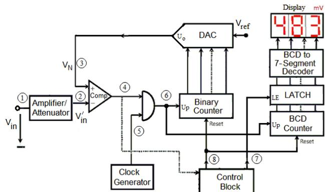
Fig. 3. Staircase digital voltmeter block diagram.
