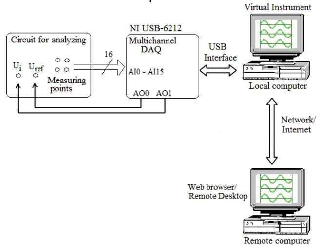
Fig. 2. Laboratory measurement using local access and remote measurement.
