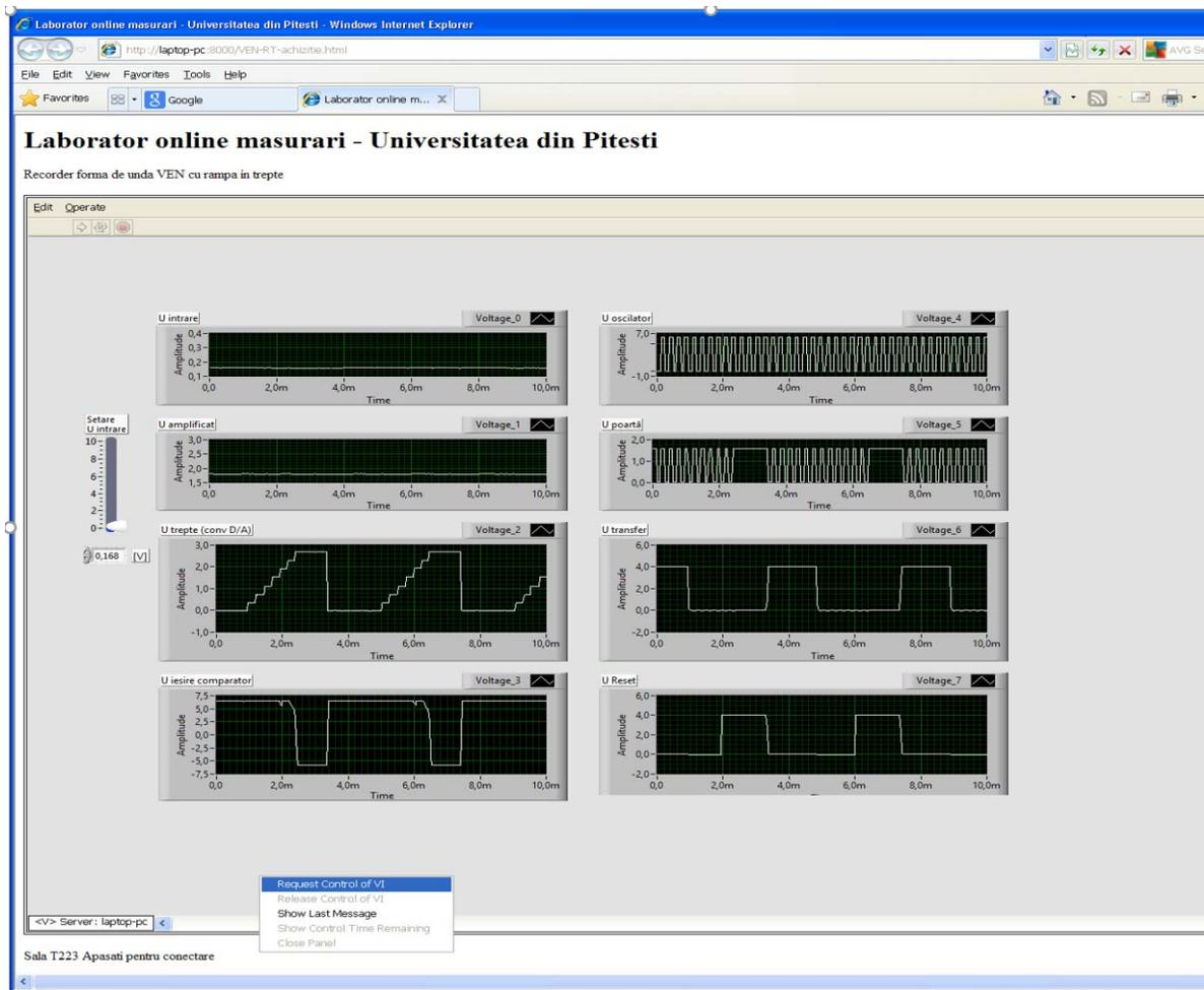
Fig. 6. Remote control of the application in web browser using Remote Desktop Connection in LabVIEW
