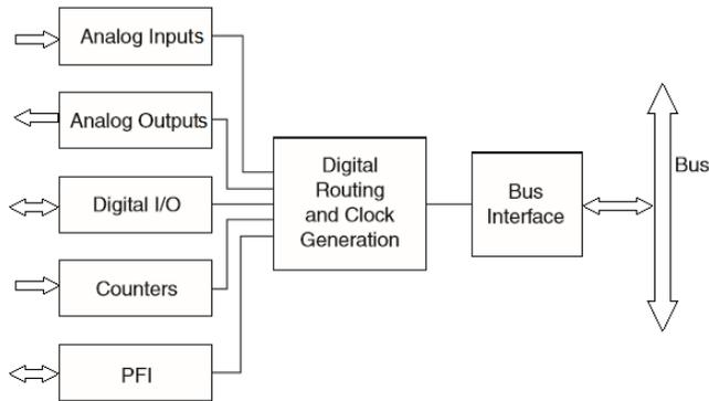
Fig. 1. Typical multifunctional DAQ module.
