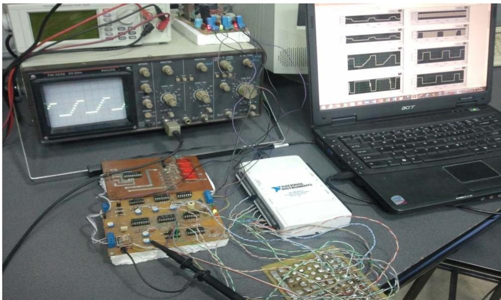
Fig. 5. Measuring waveforms in case of staircase digital voltmeter circuit and LabVIEW application.
